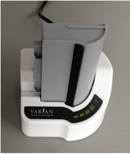
Figure 2-13 VCD Battery Pack and Charging Station
