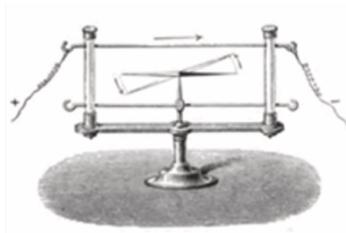
FIGURA 1. Experiment d'Oersted.
