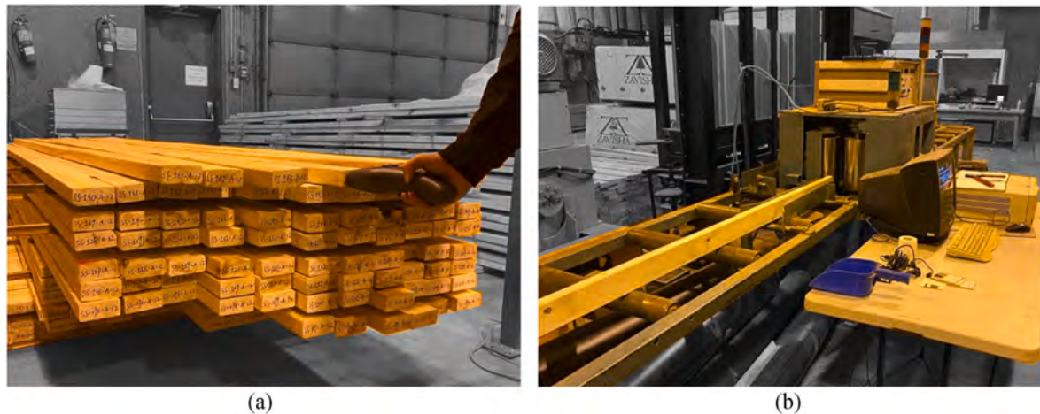
Fig. 3. (a) LSW test setup (Model: MTG-820); (b) MSR test setup (Model: Tecmach Limited Stress Grading Machine System SG-AF).
