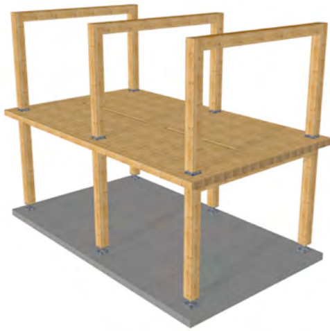
Fig. 1. Typical layout of post-beam-panel system (adapted from [9]).
