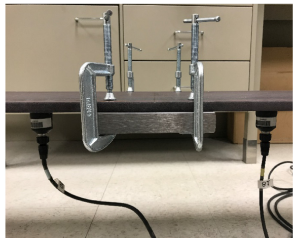
(b) DC2: Added mass at mid-span
