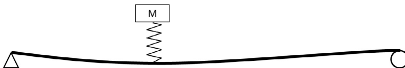
Fig. 6. Spring mass vehicle bridge interaction model (adapted from [10]).
