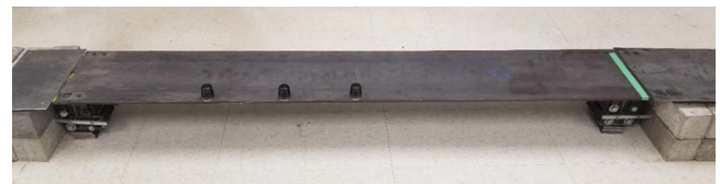
Fig. 1. Pin–roller bridge setup.
