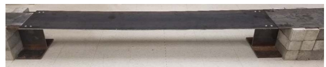
Fig. 3. Fixed–fixed bridge setup.
