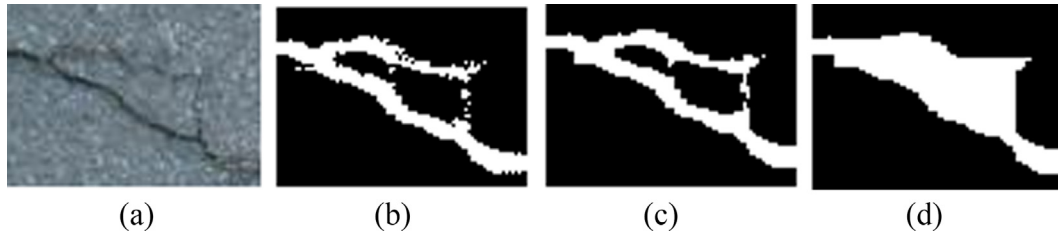
Fig. 6. Issues with deconvolution layer output (a) original patch; (b) raw output; (c) after 3 × 3 morphological operations; (d) after 15 × 15 morphological operations.
