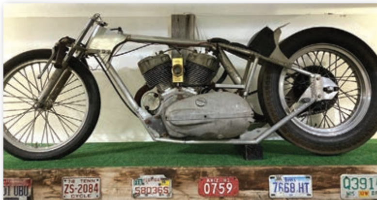
Early drag racing motorcycle. This bike was piloted by Sammy Satterlee in the early 1960's. It's powered by a Harley-Davidson K-model motor. It doesn't have a front brake and the rear slick is a recapped tire.
