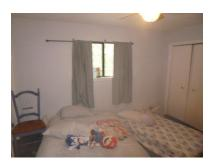
Bedroom window sills measure at a height in excess of 44" above the floor.
