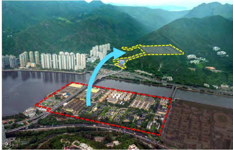
Figure 6: Relocation of Sha Tin Sewage Treatment Works (STSTW) to Caverns
