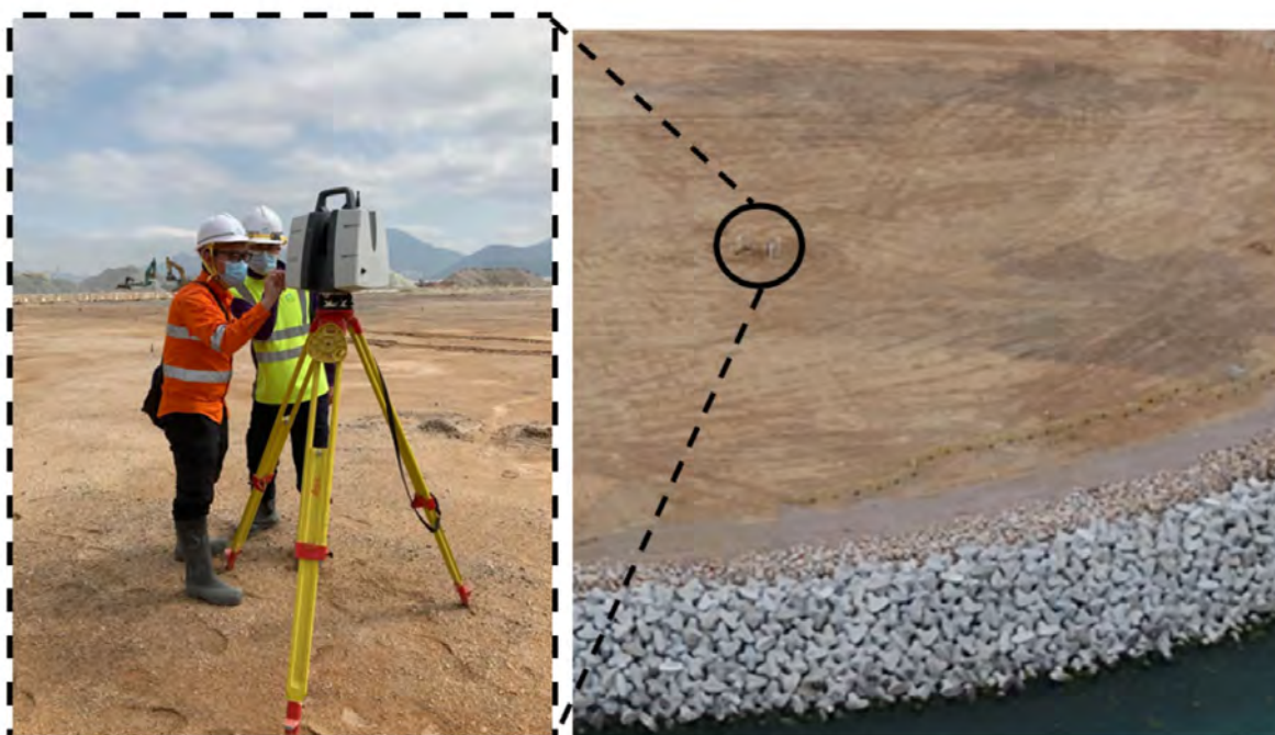
Figure 9: Typical Localised Monitoring Point Set Up for Manual Monitoring
