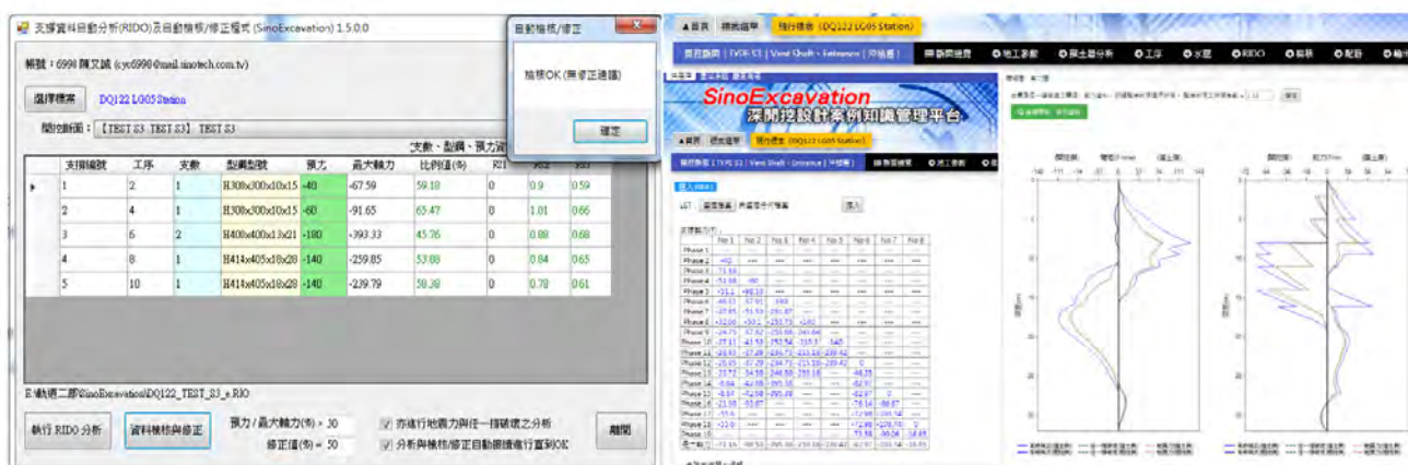
Figure 1: (Left) The Winform interface, which can automatically call RIDO to conduct the iteration itself (Right) The analytical results will be kept in SinoExcavation platform
