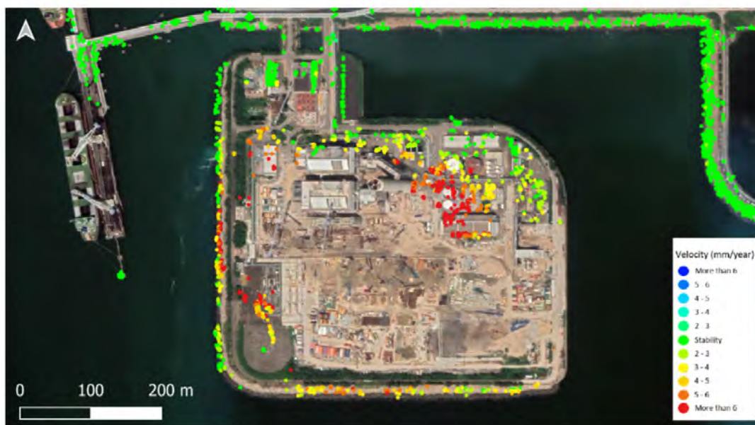
Figure 6: Velocity of deformation map in the South of Lamma Island (Hong Kong)
