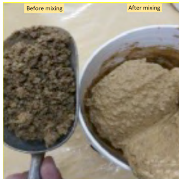
Figure 3: Soil before and after conditioning
