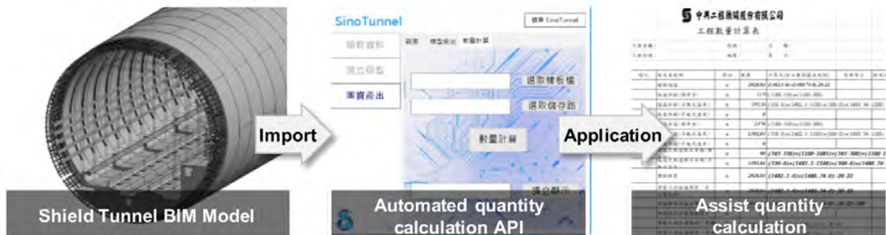
Figure 9: The process and interfaces of SinoTunnel auto-generated quantity calculation
