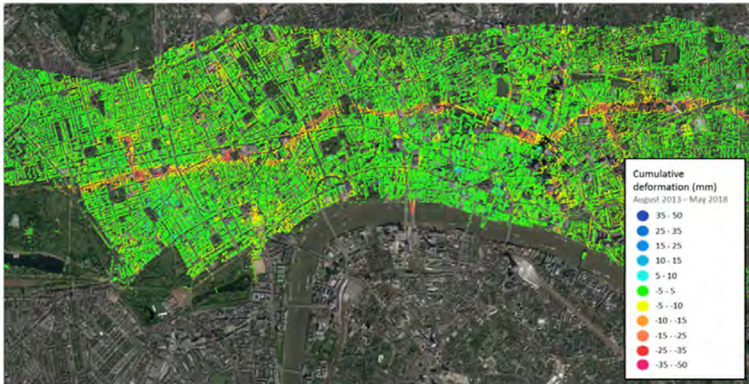
Figure 8:Accumulated deformation map over the tunnel alignment of Crossrail project (London, UK)
