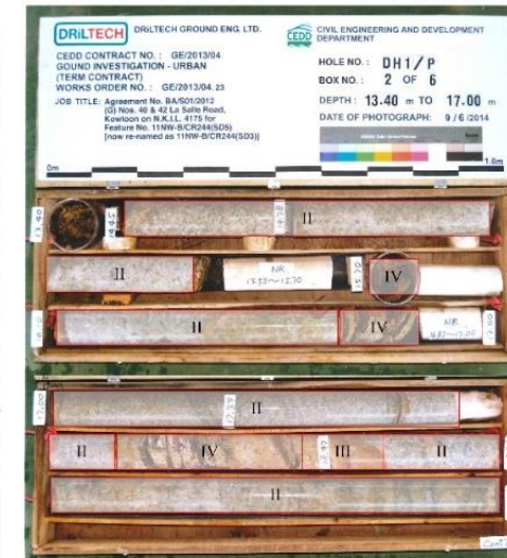
(c) original core box photo labeled with weathering grades
