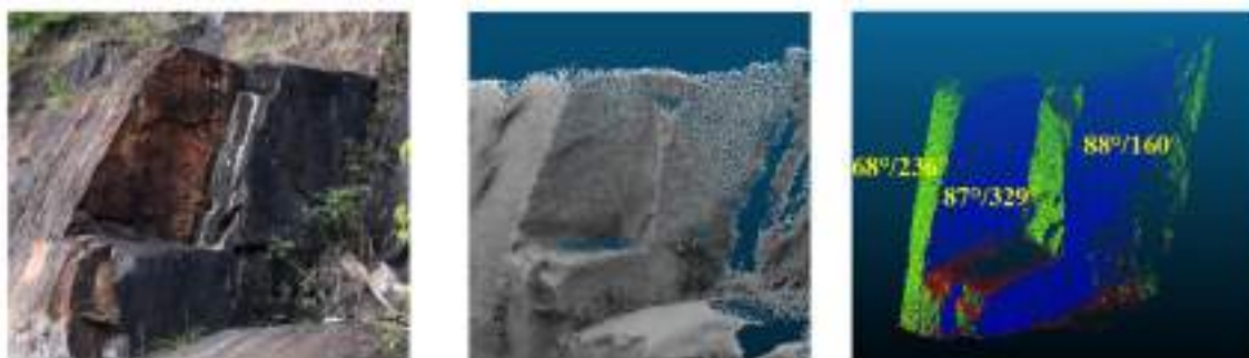
Figure 14: (left) The rock joints surveyed (middle) Point cloud data of the rock joints (right) Rock joint measurements generated by open source software
