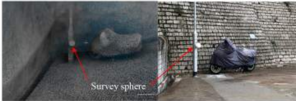
Figure 3: Geo-referencing of point cloud data can be carried out by taking the x, y coordinates and the elevation of a few targets (for example, survey spheres) on field
