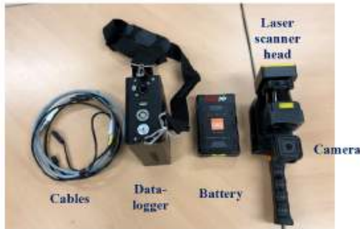
Figure 1: The HLS equipment (30 m range) used in the study
