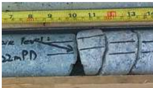
(a) Conical and Damaged Face in Concrete and Rock Cores, Drilling Breaks in Rock Cores
