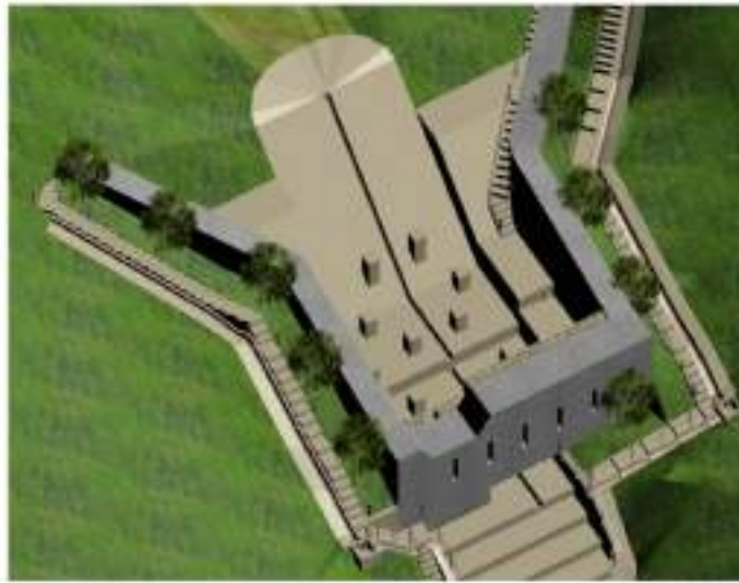
Figure 1: Debris-resisting rigid barrier BIM model
