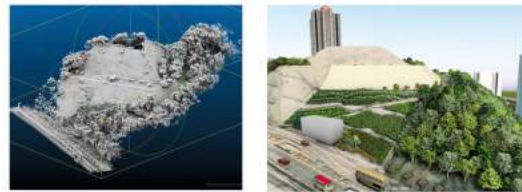
Figure 13: Point cloud data of existing site conditions collected by HLS (left) and visualisation of design options in BIM (right)
