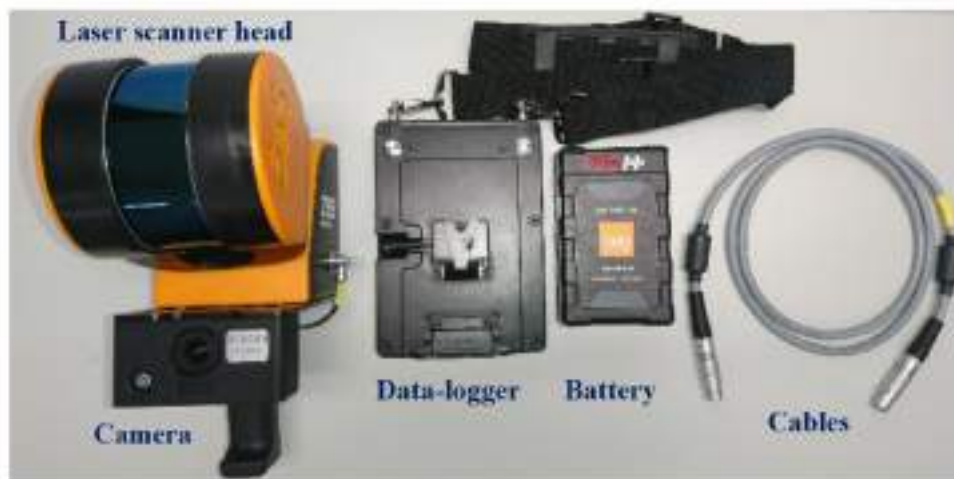
Figure 2: Another new model of HLS equipment (100 m range) used in the study
