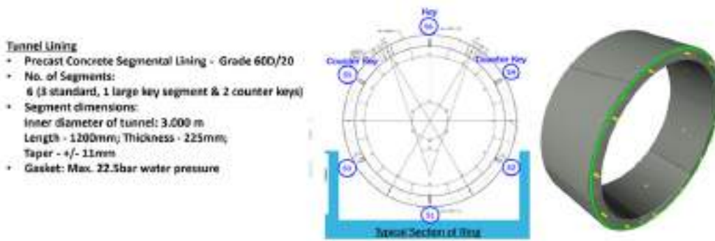
Figure 1.6: Precast Concrete Segment Ring
