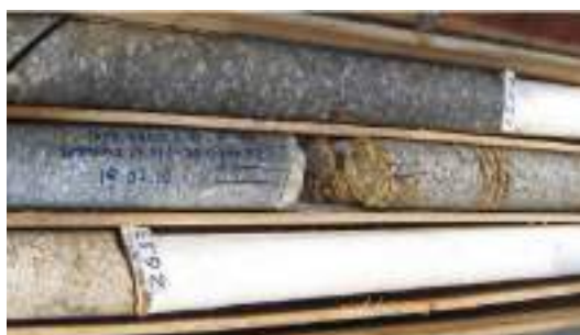
(a) Weak Seams at Interface and in Rock Core
