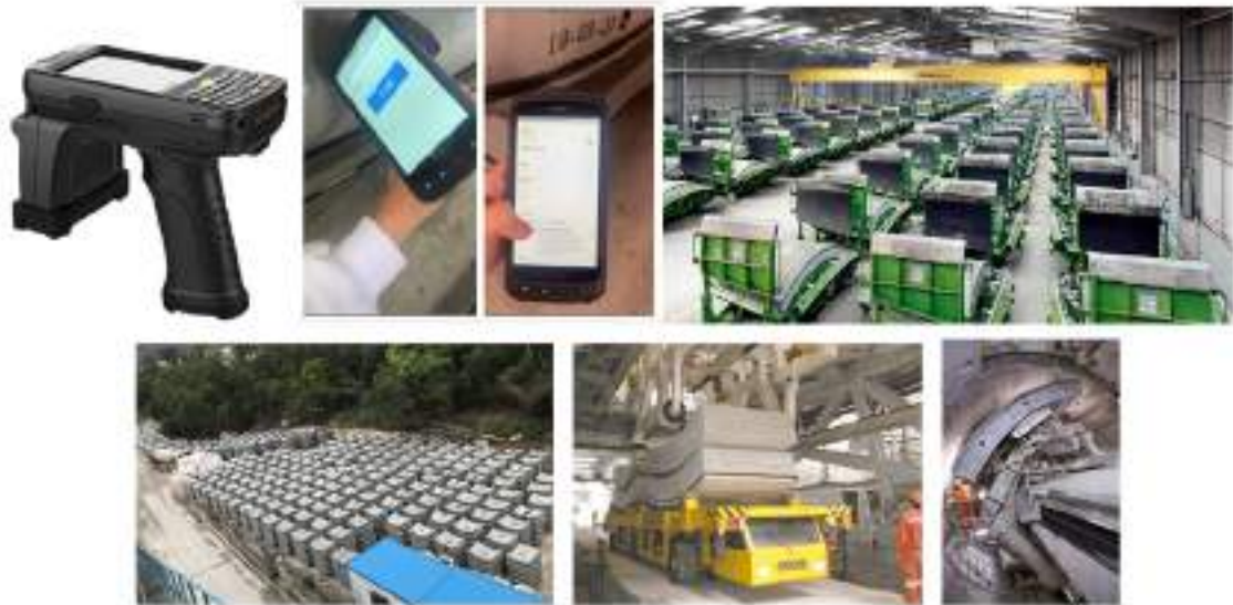
Plate 3.4: RFID Scanning by the Handheld Reader from Precast Segment Storage Yard to IRTS Site
