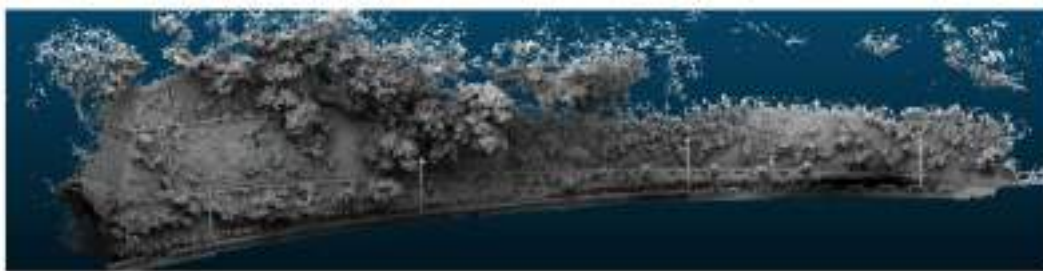
Figure 6: Point cloud data taken at Feature No. 11NW-D/C90 under moderate rain (daytime)
