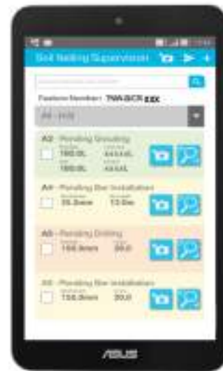
Figure 3: Mobile App displays the details of soil nail schedule
