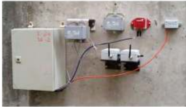
Plate 9: Tilt sensor comparison test
