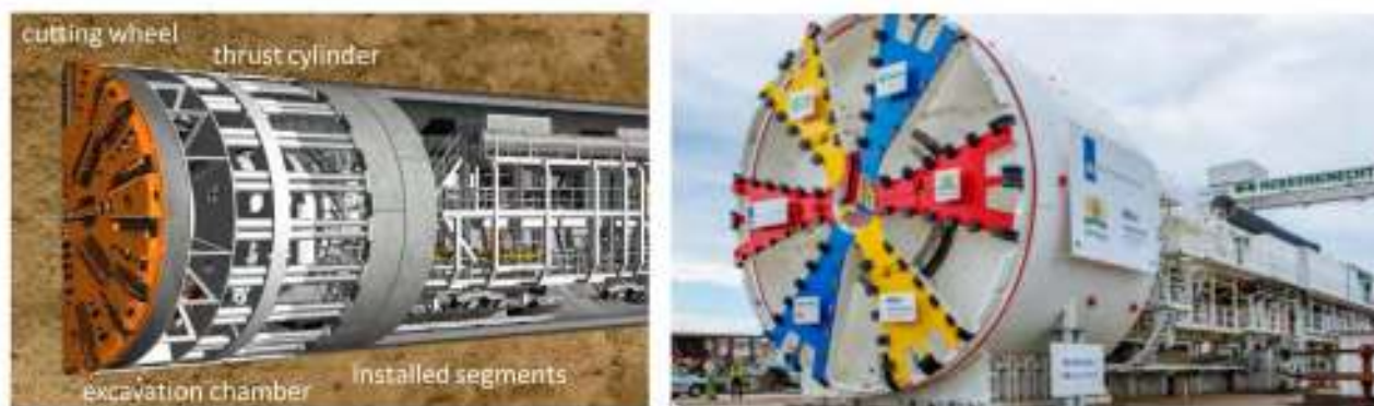
Figure 2: (left) Tunnel Boring Machine (courtesy of Herrenknecht); (right) the Rotterdamsebaan Tunnel Boring Machine (courtesy of Municipality of The Hague)
