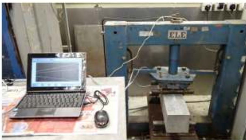
Figure 4: SFRC beam flexural testing
