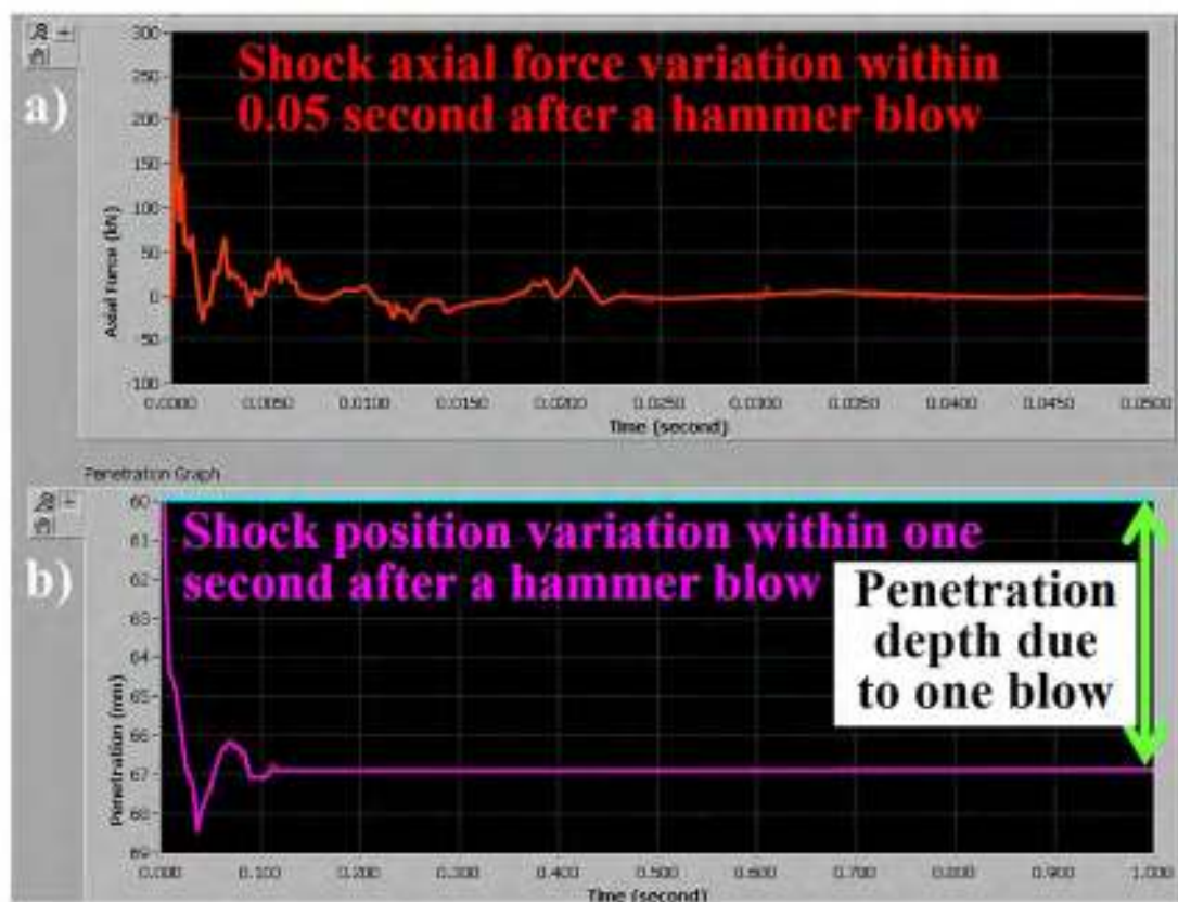
Plate 6: The measured results of the automatic SPT N-value Monitor by one hammer blow at field
