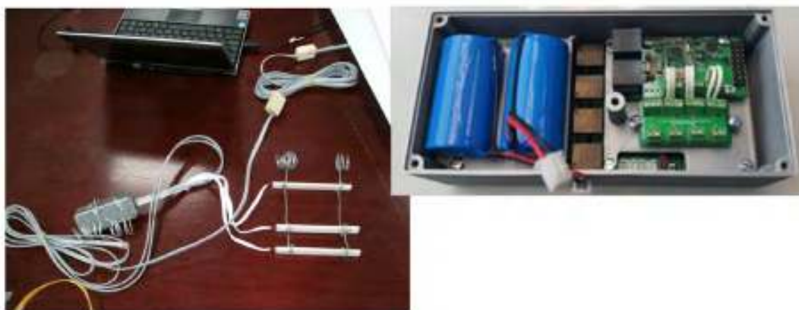
Figure 1: Foil strain gauges and strain gauge module (SGM), Figure 2: Data logging module (DLM)
