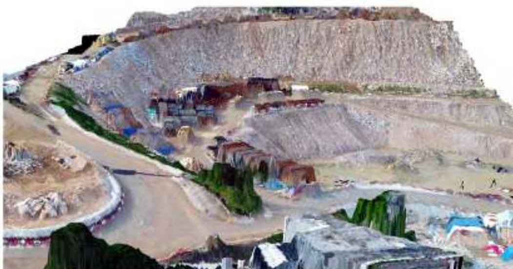
Figure 3: An example of DTM and orthomosaic image created by drone photogrammetry
