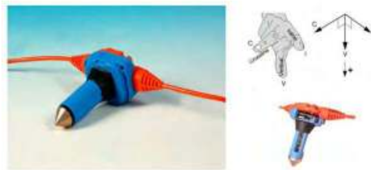
Figure 7: MEMS receiver technology allows simultaneous capture of seismic information along three axes and from very low to very high frequencies and opens up the opportunity for simultaneous imaging of structure and geotechnical conditions (Source: Sercel).
