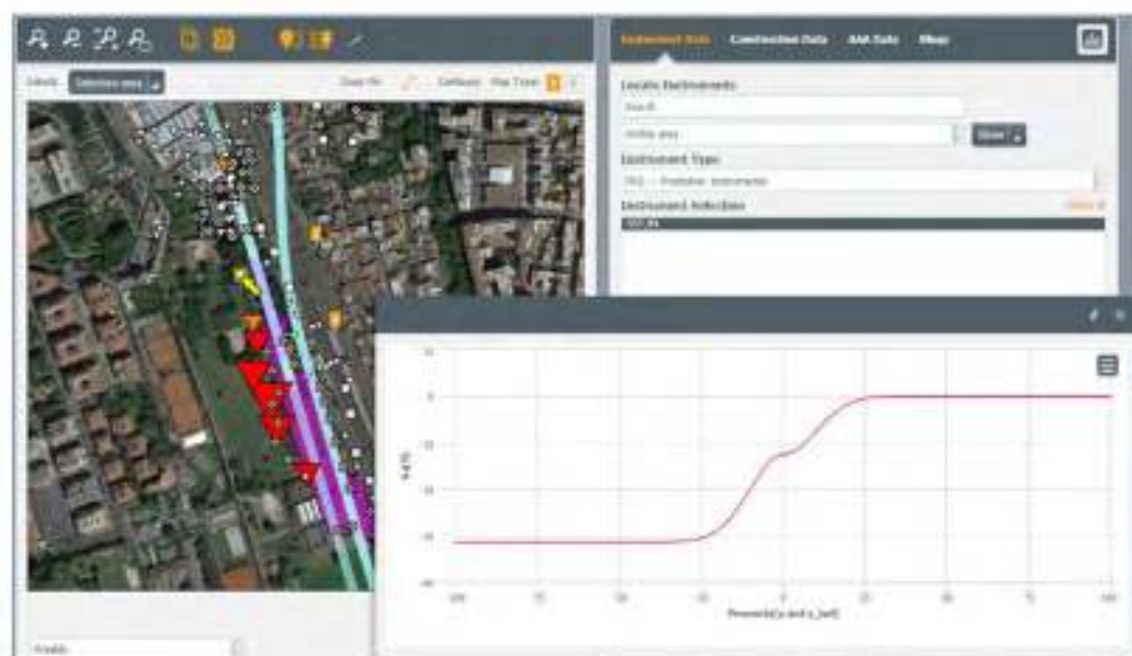
Figure 11: Proximity based dynamic prediction of settlement.
