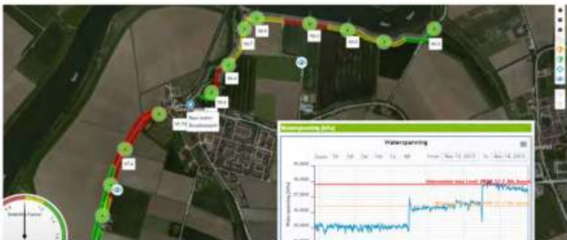
Figure 9: Gaia Insight – excess pore pressure as indicator for reduced slope stability during construction
