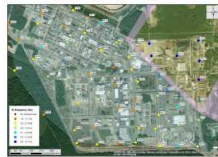
Figure 13: H/V microzonation is highly suited to industrial or urban environments. In this example f_0 frequencies were acquired over a major industrial site. (Source: Fugro).
