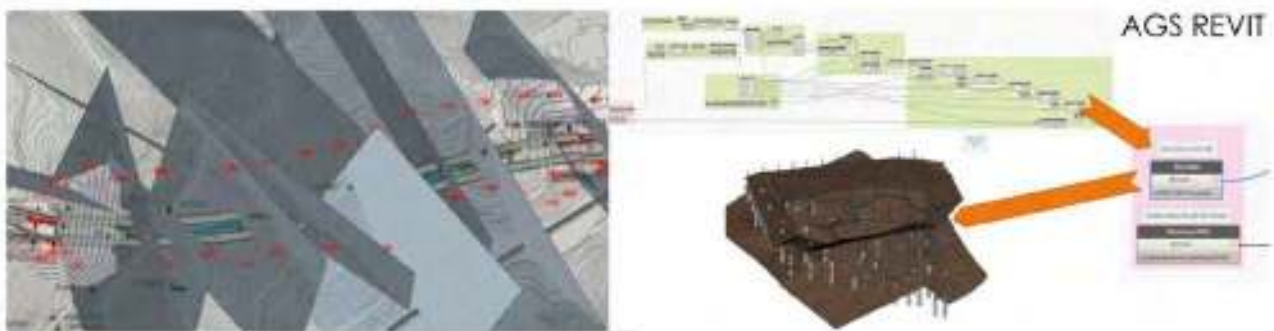
Figure 2: Parametric 3D modeling directly from AGS
