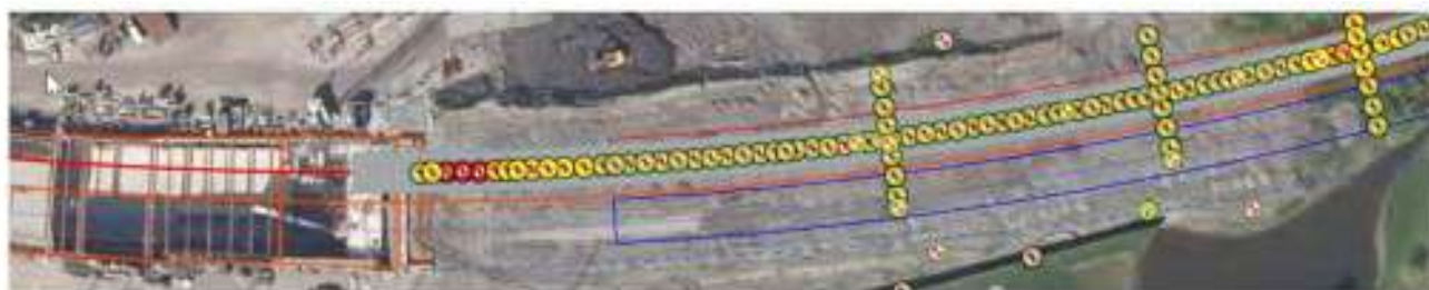
Figure 5: Overview of the Gaia Insight Decision Support Platform: the start shaft tunnel, the dotted lines indicate the predicted surface settlements, and the red, yellow and green icons indicate prism locations and surface settlement.
