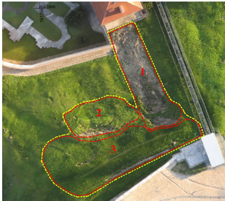
Figure 11: Landslide area in spring 2016 (Lithuaniae Academia Scientiarum 2016): 1 – landslide area ( 351 \text{ m}^2 ); 2 – slope deformations and possible ensuing landslide area ( 222 \text{ m}^2 ); 3 – slope deformations and possible ensuing landslide area ( 645 \text{ m}^2 ).
