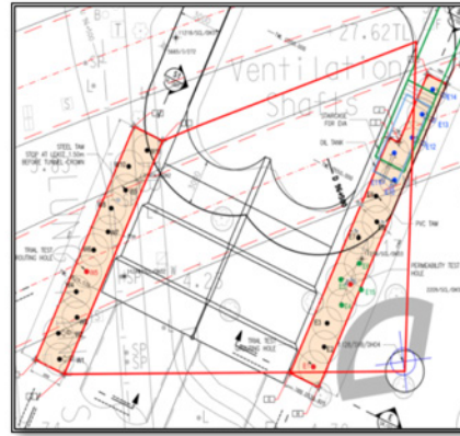
Figure 8: Vertical TAM grouting Layout
