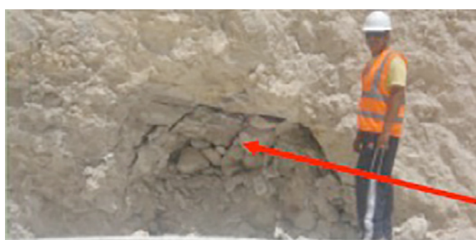
Figures 11 and 12: Karst identified in the Simsima Limestone, immediately above the Midris Shale boundary
