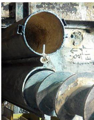
Plate 6: O-pile system for a tunneling project in HK (Courtesy of Mincon Group)
