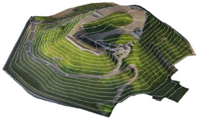
Figure 12: Gediminas Hill topographical monitoring (Lithuaniae Academia Scientiarum 2016): on the left hand – digital topography scheme; on the right hand – digital surface (2.5-D view)
