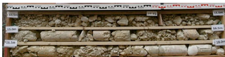
Figure 10: Simsima Limestone, intense karst weathering, MQD V
