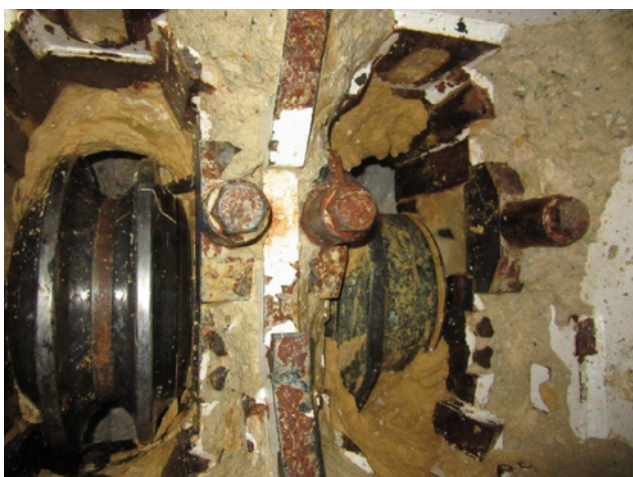
Figure 27: Cutter clogging with clay (Midris Shale)
