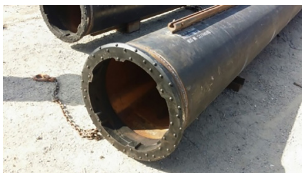
Plate 5: A Mincon ring bit connected to pipe pile
