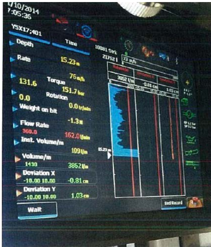
Plate 3: Screen of Real-time monitoring of CSM parameters
