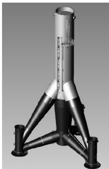
(a) Piled tripod structure (Merritt et al. 2012)
