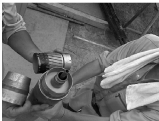
Plate 3: Gel-Push triple tube sampler coats the sample in a gel for frictionless recovery of samples.
