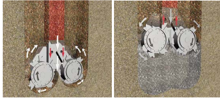
Figure 1: Construction process in Geomix technique with CSM equipment [1]
