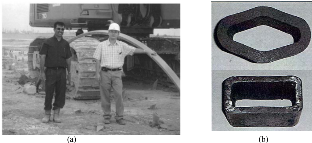
Figure 4: (a) A Bent Mandrel (b) Common cross-sections of mandrels (after Bo and Choa 2004)
