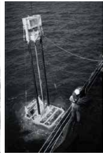
Plate 3: Vibro-core piston sample
