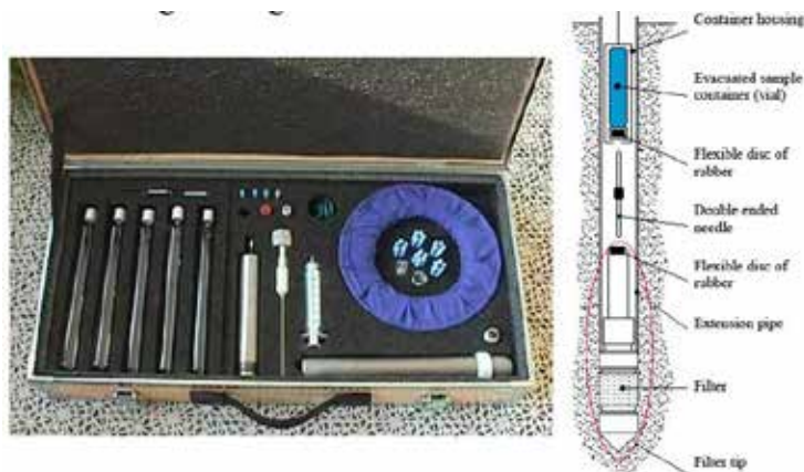
Plate 2: GeoN groundwater gas sampler
