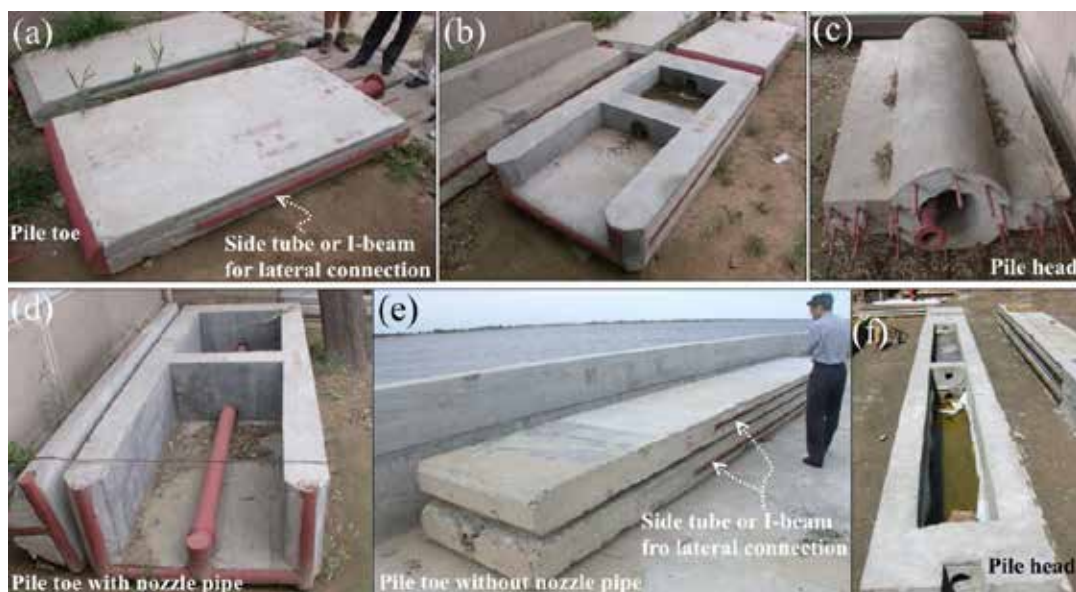
Figure 2: Various and flexible design of precast reinforced concrete piles for jetting and grouting installation
