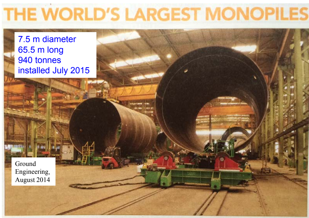
Figure 8: Photograph of 7.5 m diameter monopiles for the Gode Wind farm
