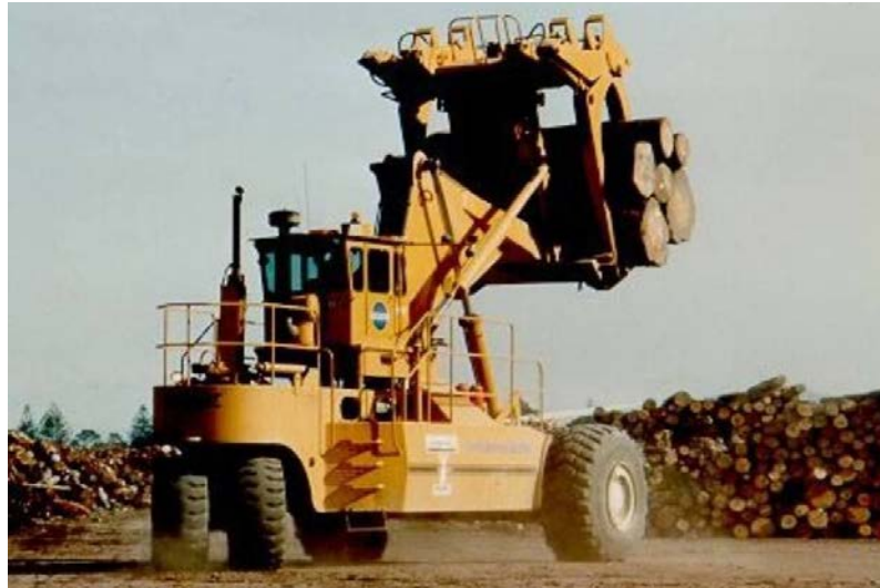
Figure 8: Log handling Wagener operating on new construction
