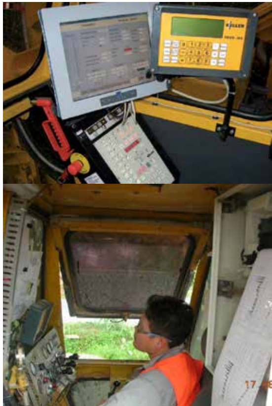
Figure 5: Rig operator's control and display units
