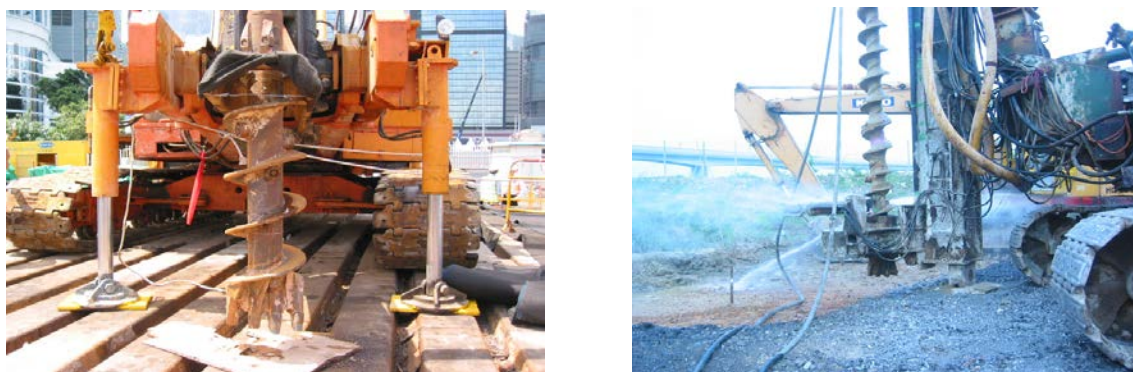
Figure 1: The nozzles mounted at the tip of the auger stem
