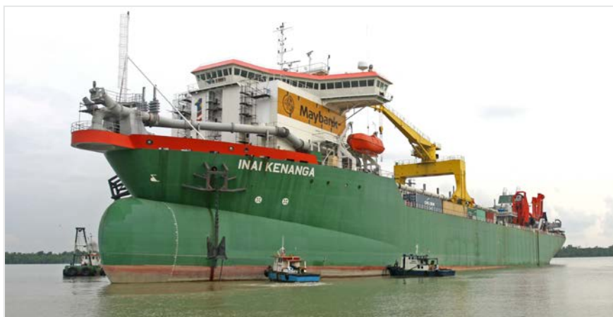
Figure 23: Trailing suction hopper dredger “Inai Kenanga”, owned by IMW Malaysia
