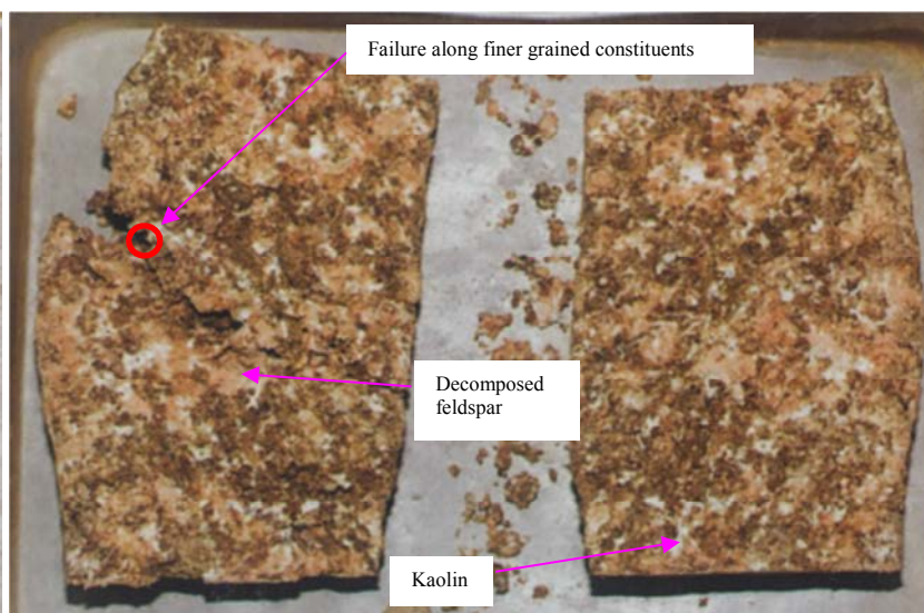
Plate 6: Specimen 3 - Failure Cut Section
