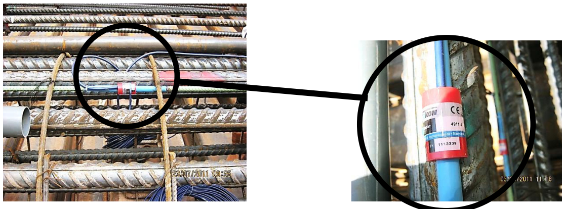
Plate 11: Vibrating wire strain gauge attached to sister bar inside the trial pile
