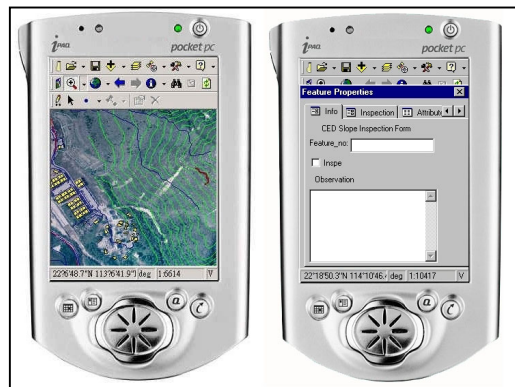
Figure 8 - Field information can be recorded as GIS data (left) and on customized form (right).
