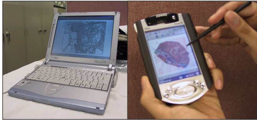
Figure 4 - Hand-held (left) and pocket (right) computer equipped with GIS software and Bluetooth technology.
