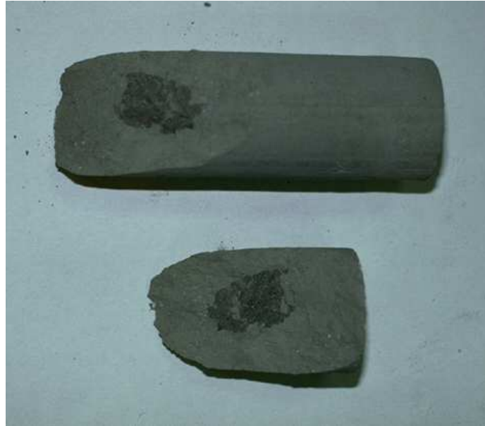
Figure 3.5. A RCTS sample with a shear plane after a TC test, Sagamihara test site.
