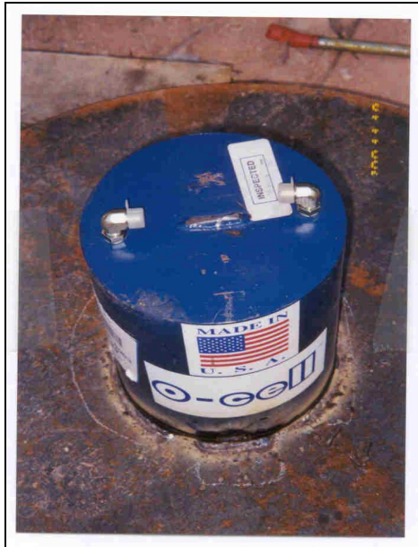
Figure 5A – 230 mm-dia. Osterberg Load Cell
