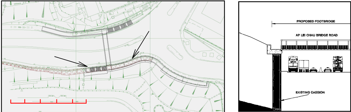
Figure 15 : Retaining wall layout and section under revised scheme
