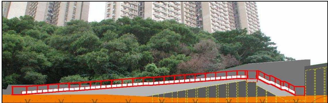
Figure 15 : Retaining wall layout and section under revised scheme
