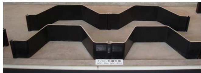
Figure 1(b): Photo of Hat-type sheetpile
