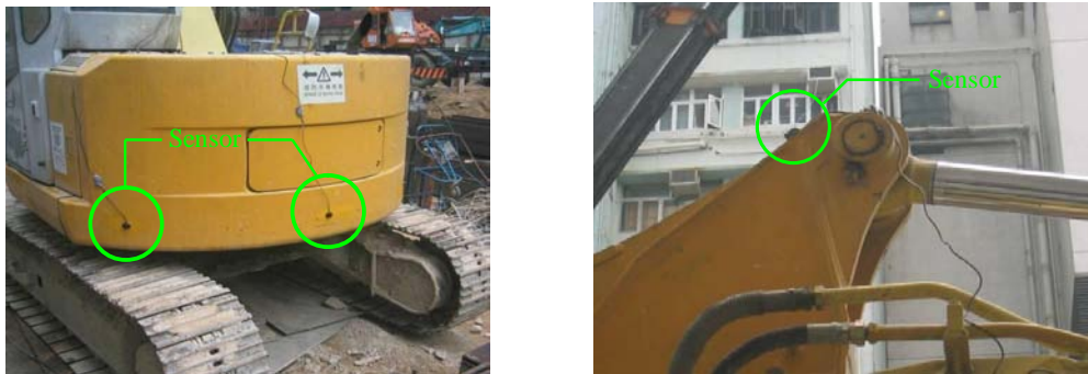
Figure 7: Distance sensors mounted at the rear (left) and at the arms (right) of backhoe
