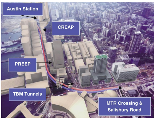
Figure 1: Kowloon Southern Link alignment.
