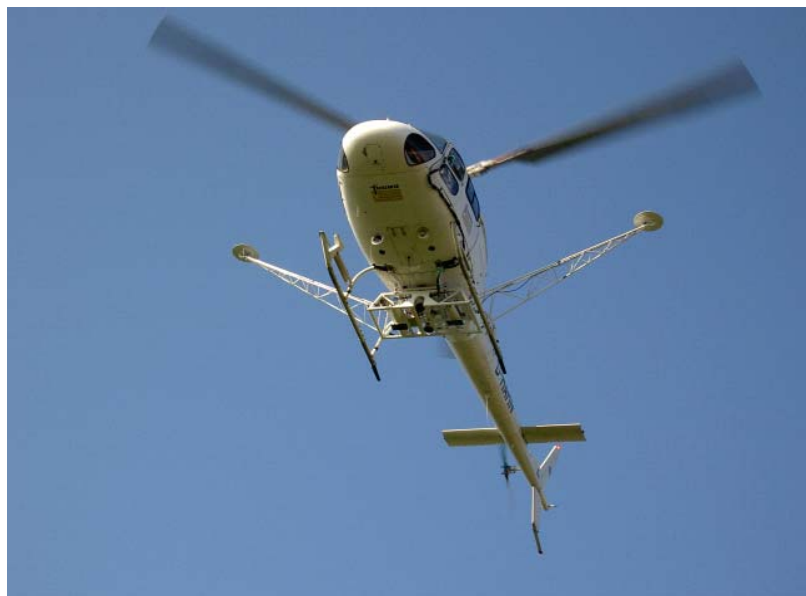
Figure 8: FLI-MAP LiDAR system mounted below a helicopter (photo courtesy of Fugro Aerial Mapping BV)
