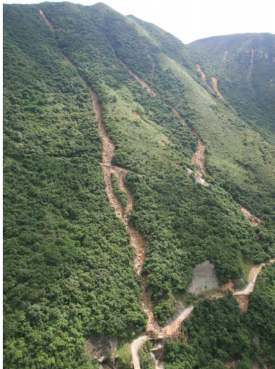
Figure 30: Debris flow with significant entrainment in the June 2008 rainstorm (Note: Debris flow above Shum Wat Road is shown; the source volume is less than 100 \text{ m}^3 and the entrainment ratio exceeds 10)
