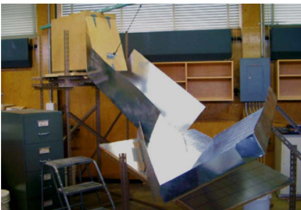
(a) Laboratory apparatus used for deflected sand flow tests (after Pudasaini & Hutter 2007)
