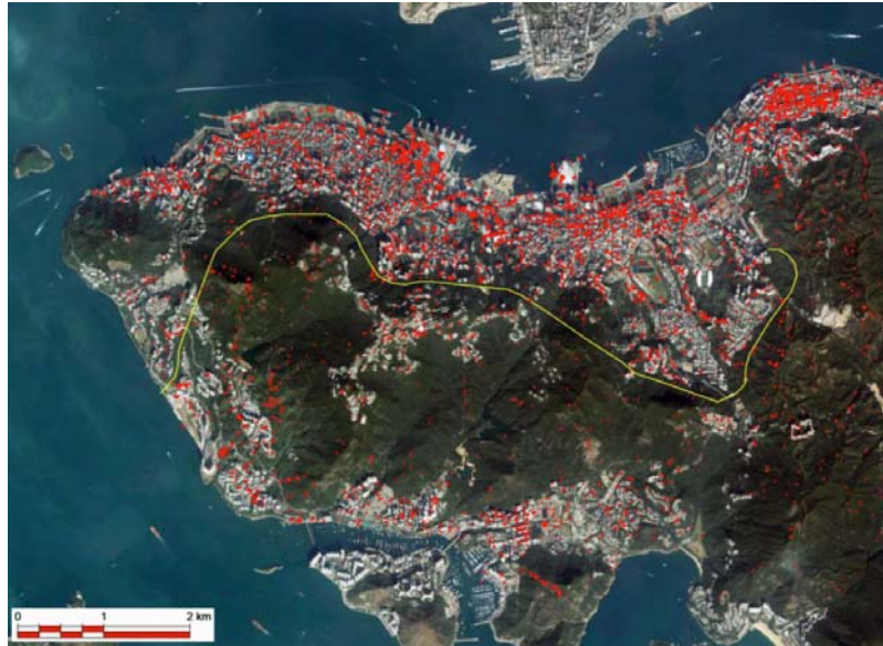
Figure 3: Location of persistent scatterers on Hong Kong Island (image courtesy Fugro NPA Ltd)
