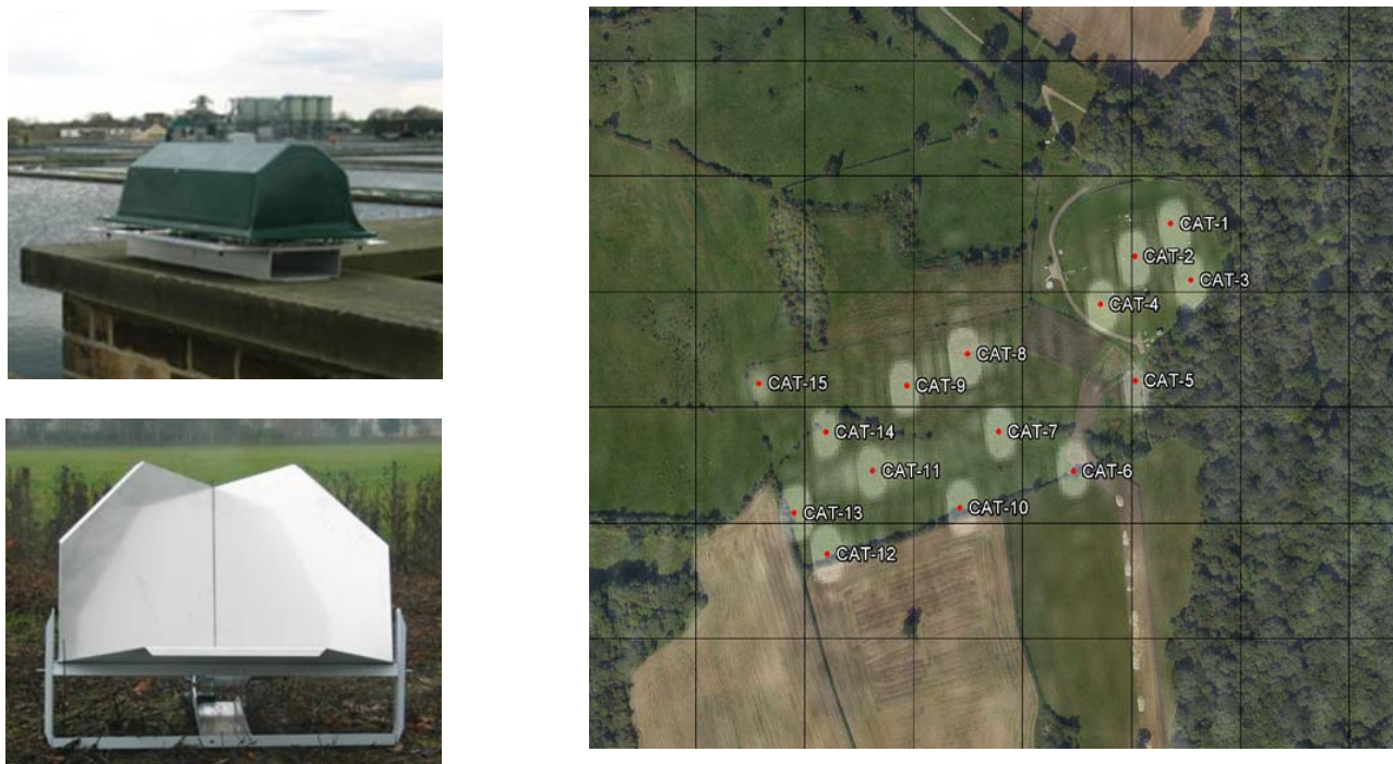
Figure 5: (clockwise from bottom left): Corner reflector (CR); Compact active transponder (CAT); CAT responses in SAR image (all images courtesy Fugro NPA Ltd)
