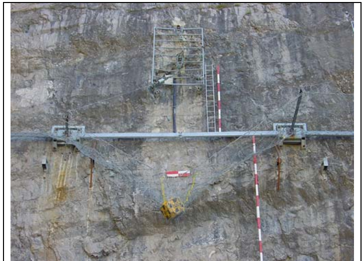
Plate 3: Testing Isostop 250 kJ system in Walenstadt
