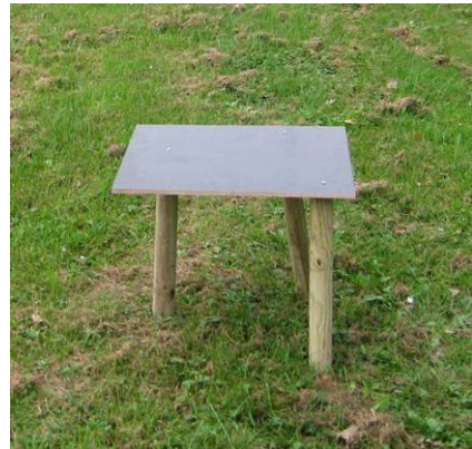
Figure 7: LiDAR marker board
