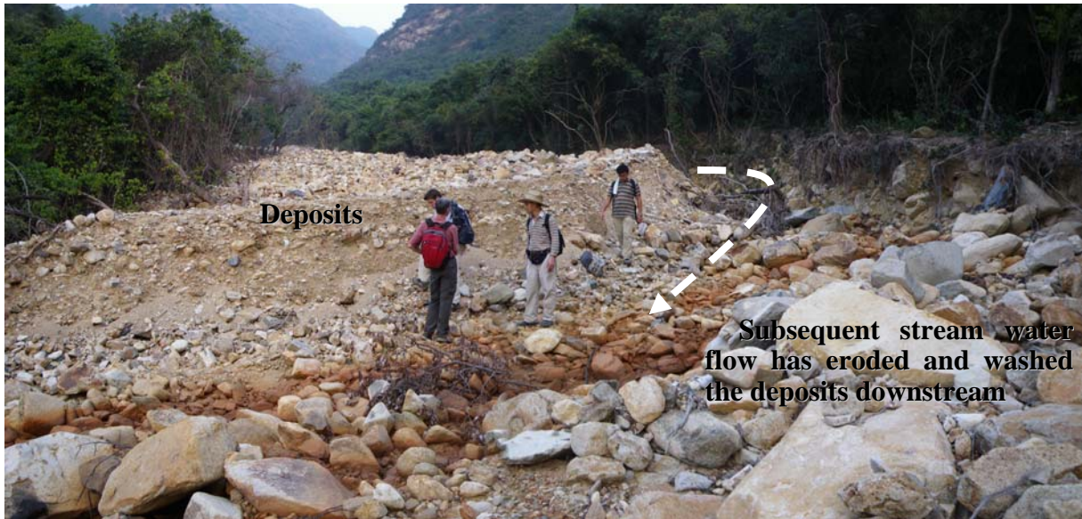
Figure 28: Deposits of a watery debris flow at the deposition zone (Note: The June 2008 Shek Pik No. 4 debris flow is shown; the deposits have been subject to considerable sorting)
