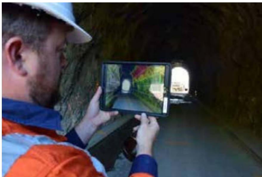
Figure 14: Augmented reality on 3D laser scanning of tunnel profile.
