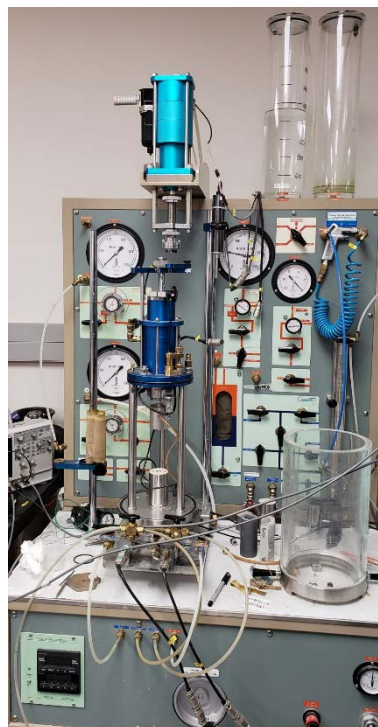
Figure 29: Torsional shear testing setup.
