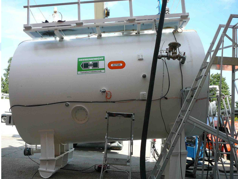
Figure 11 Pressure chamber for shotcrete trial
