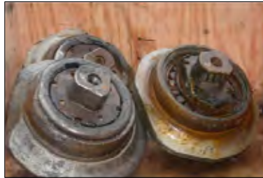
Damaged disc cutters
