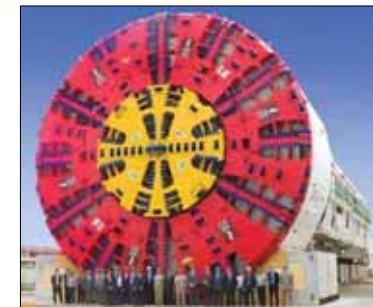
Herrenknecht 15.2m OD TBM Madrid: gypsum, soft rock
