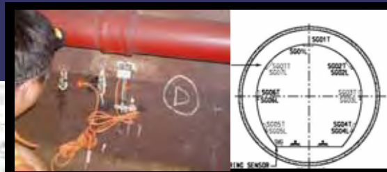
84 strain gauges + seismographs
