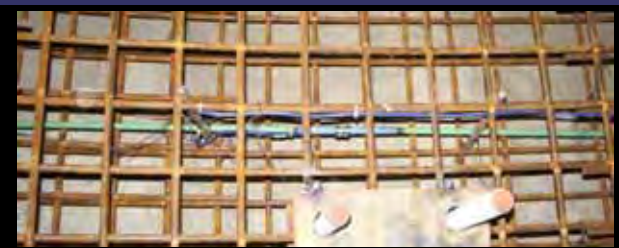
sister bar embedded in concrete ring beam
