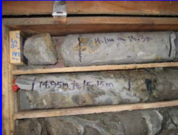
T.A.M. Grout Core Sample
