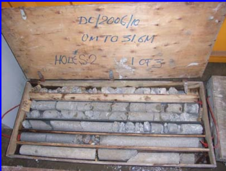
Jet Grout Core Sample
