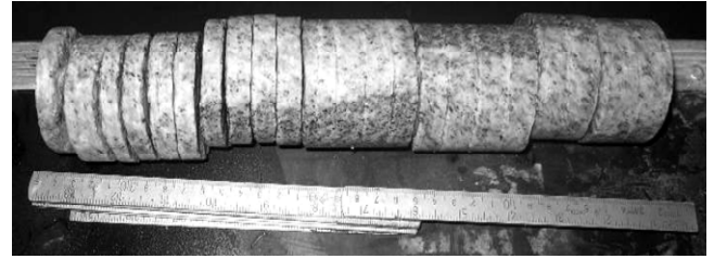
Fig. 21 Illustration of Core dishing: 23 Disks Observed in a 27 cm Long Core [LU et al, 2011])
