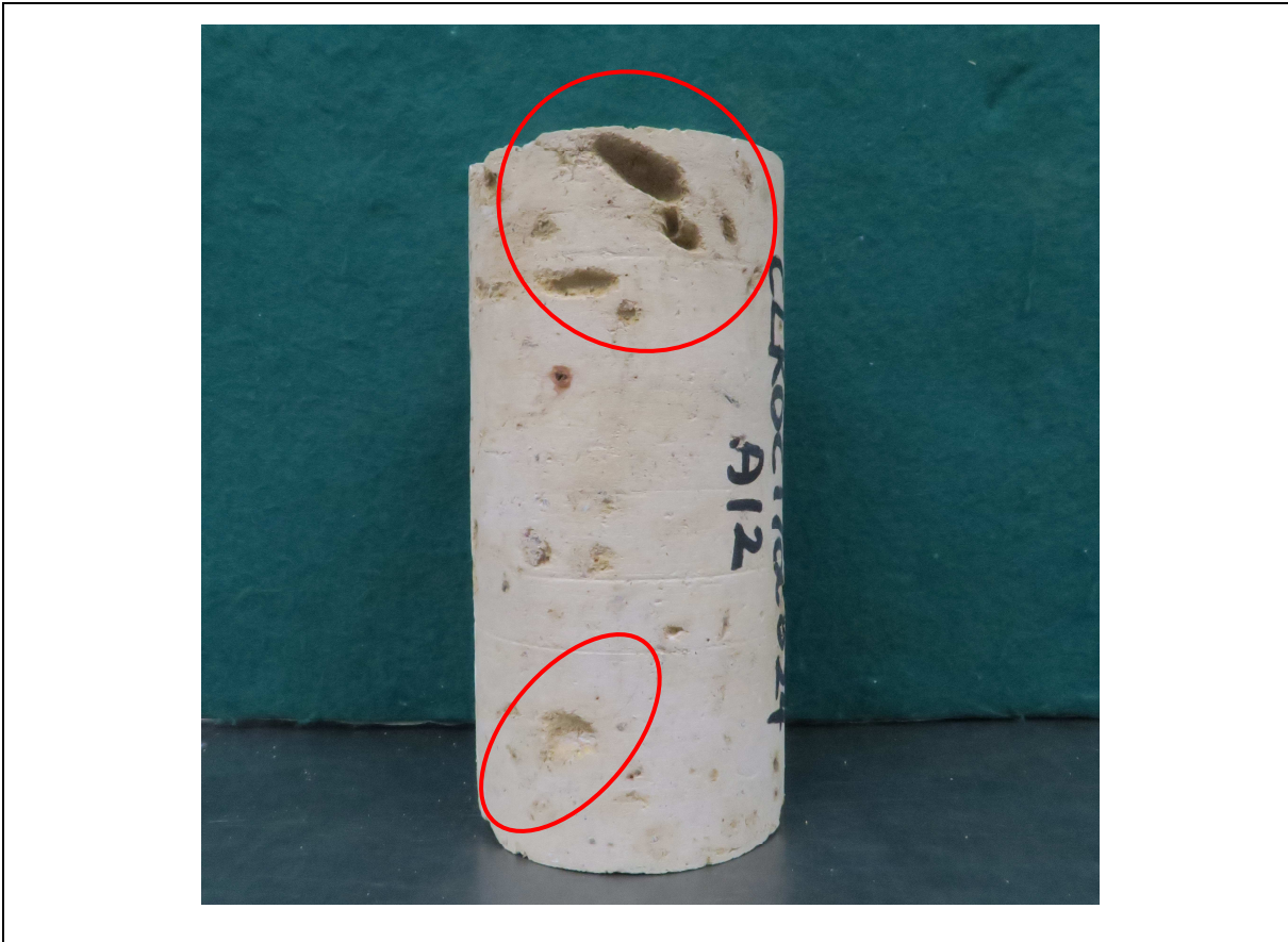
Figure 9 Soft Spots on Cement Stabilised Soil Specimen
