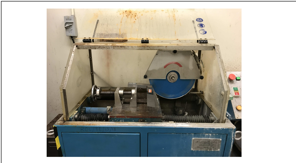
Figure 7 General Set-up of Rock Saw (Photo Credit: Public Works Central Laboratory, CEDD)
