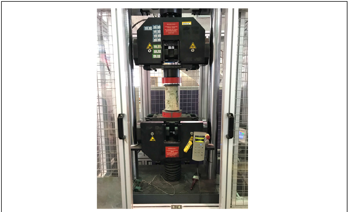
Figure 6 General View of UTM Machine (Photo Credit: Public Works Central Laboratory, CEDD)
