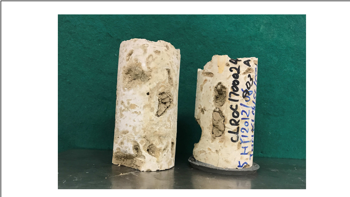
Figure 10 Voids and Soft Spots on Received Cement Stabilised Soil Cores
