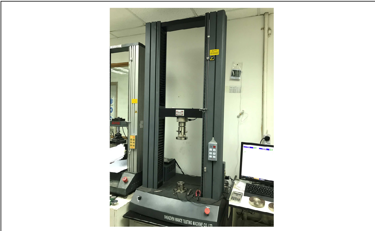
Figure 3 Example of Load Frame (Photo Credit: Quality Control Consultants Ltd.)
