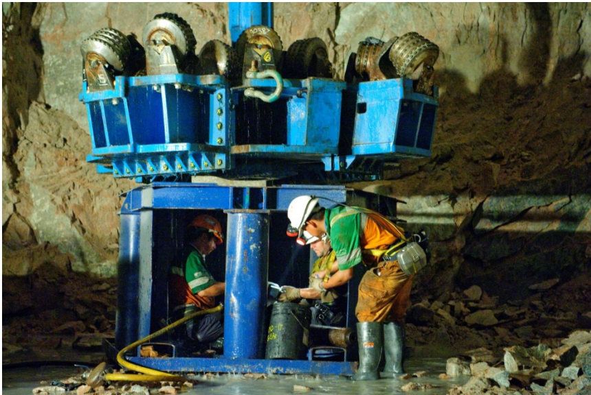
A close-up view of the reamer cutter head (courtesy of Dragages Hong Kong Ltd)
