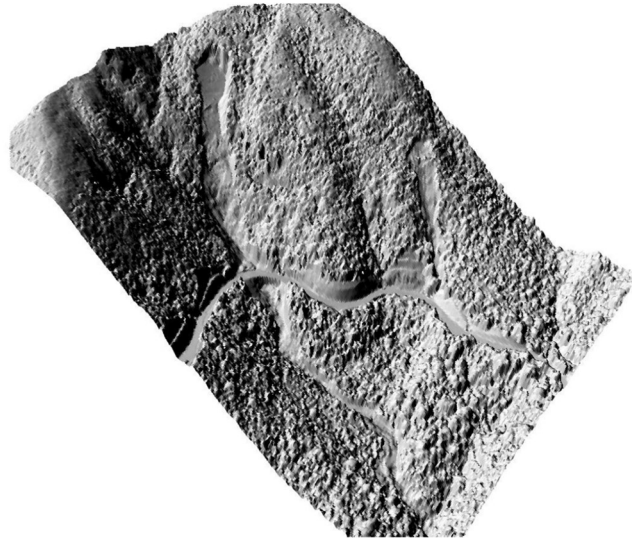
Left: UAV images of the landslide. Right: DEM generated by photogrammetry from the UAV images, which was used to assess the landslide source volume by comparison with the pre-landslide LiDAR survey data (courtesy of Geotechnical Engineering Office, HKSAR Government)
