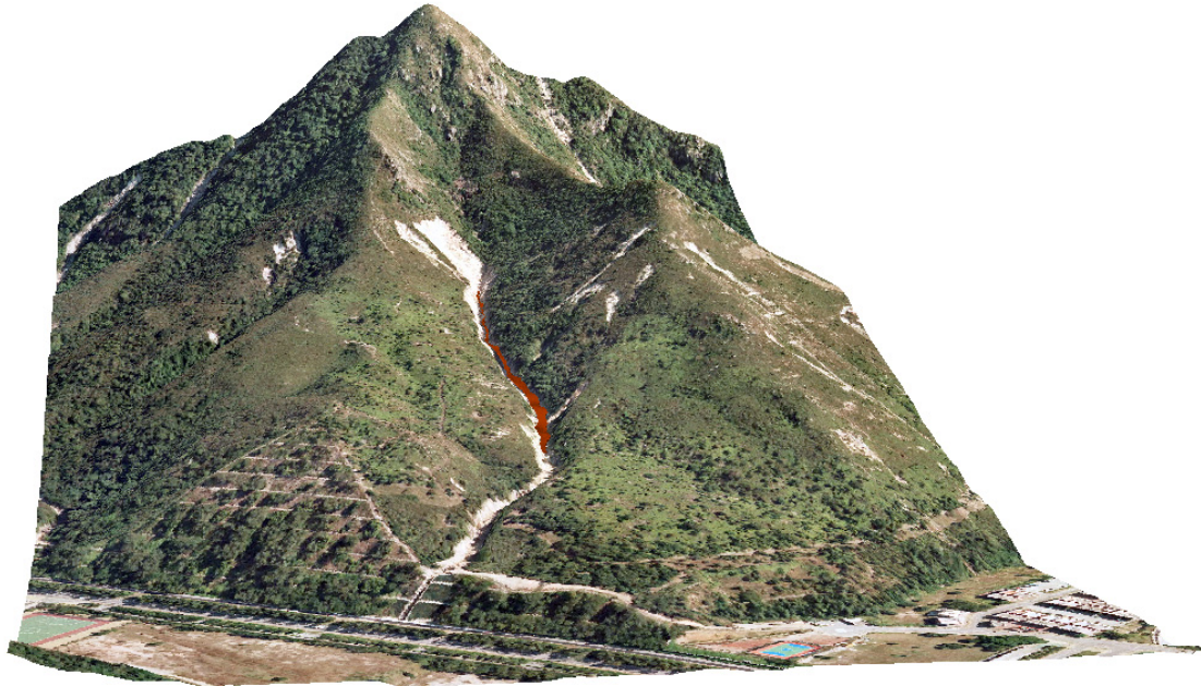
Three-dimensional debris mobility modelling of a debris flow (courtesy of Geotechnical Engineering Office, HKSAR Government)
