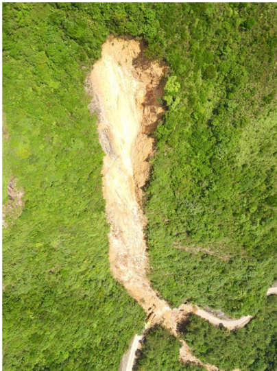
Left: UAV images of the landslide. Right: DEM generated by photogrammetry from the UAV images, which was used to assess the landslide source volume by comparison with the pre-landslide LiDAR survey data (courtesy of Geotechnical Engineering Office, HKSAR Government)
