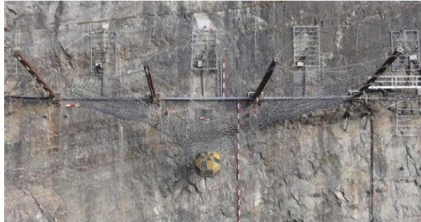
0 Front view of the falling rock protection barrier GBE-8000A after MEL test (29.11.2011).
