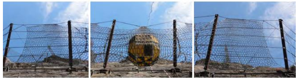
1 Bottom view of the falling rock protection barrier GBE-8000A after MEL test.
