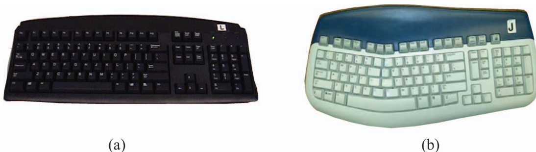
Figure 2. (a) The straight keyboard and (b) one of the curved keyboard models ( 10^\circ split angle shown) tested in Experiment 1.
