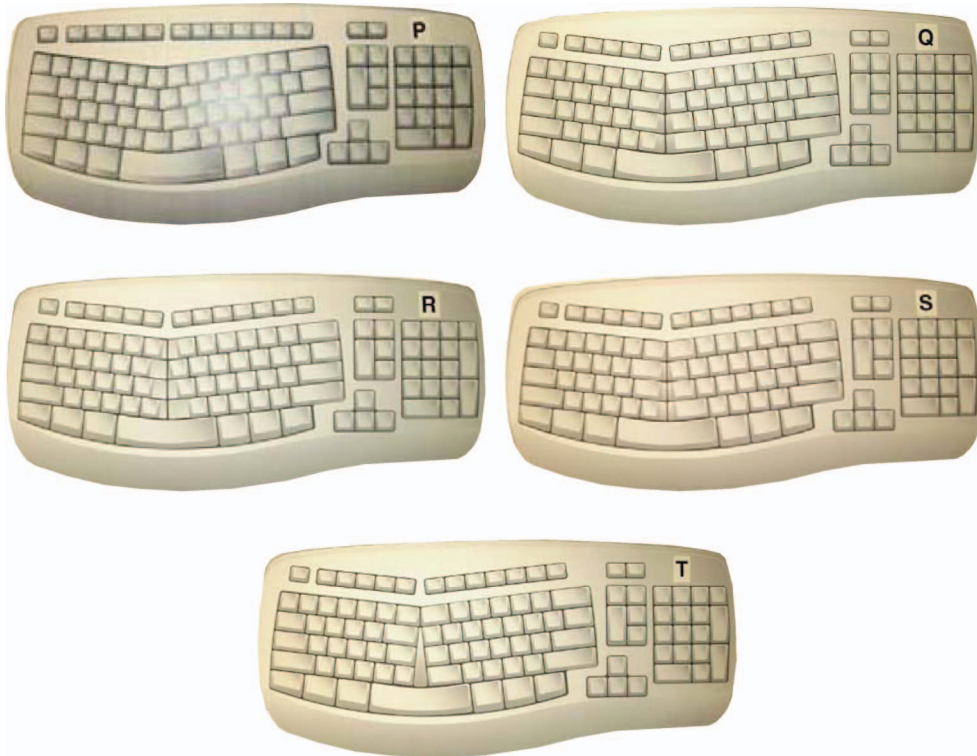
Figure 3. The non-electrically functional prototype curved keyboard models with the five alternative centre keycap designs assessed in Experiment 2.
