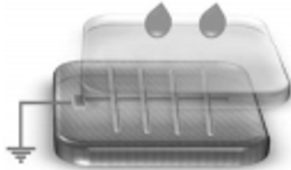
Gambar 2. Hybrid Energy Harvesting Solar Cell with Triboelectric Nanogenerator via Mutual Electrode
