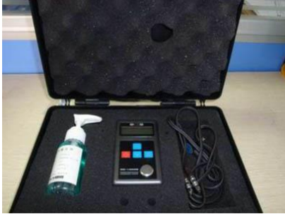
Idler steel tube thickness measuring
