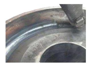
The conveyor pulley shells are one-piece rolled with single seam weld. The fabrication is accurate in concentricity. All of the shells are static balanced and can be dynamic balanced if required. All conveyor pulley shells are seam welded by MIG process. Continuous wire feeds are employed during the welding process, utilizing an inert gas atmosphere, which guarantees the maximum uniformity and resistance of weld.
