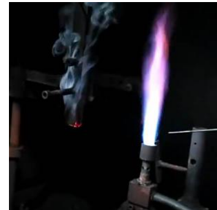
The flame goes out within 10 seconds after leaving the fire
