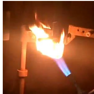
Put six individual samples of the belt on a naked flame
