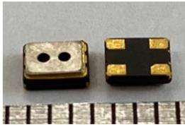
**RSM411** requires a heater power consumption of only 45mW, and is suitable for low-power equipment and battery-operated instruments. In the presence of detectable gas, sensor conductivity increases depending on gas concentration in the air. A simple electrical circuit can convert the change in conductivity to an output signal which corresponds to the gas concentration.
