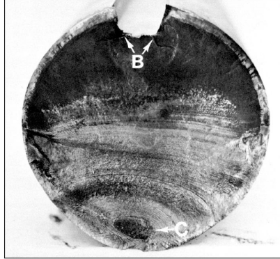
Fatigue fracture of an AISI 4320 drive shaft. The fatigue failure initiated at the end of the keyway at points B and progressed to final rupture at C . The final rupture zone is small, indicating that loads were low.
