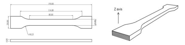
FLEXURAL TESTING SPECIMEN ISO 178, GB/T 9341
