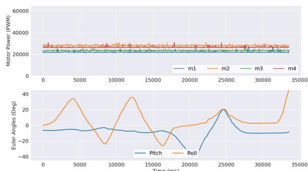
Fig. 12: Quadrotor PWM response to Euler angle disturbances with the TSAC policy. The PWMs do not respond in a way to fly, but in an exploitative manner of the dynamics model to maximize reward.
