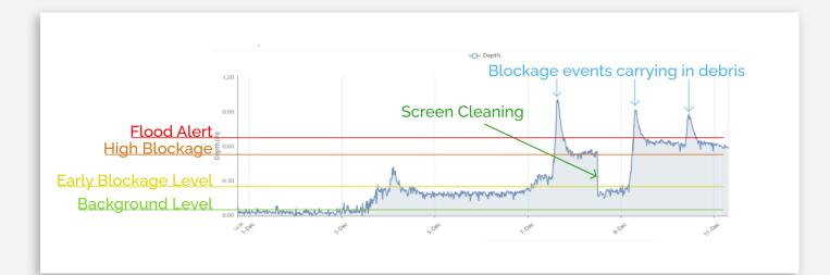
Data is easily viewable and downloadable from the UDlive Portal from any internet connected device, allowing you to clearly follow blockage trends and set up alarms. This helps you efficiently manage operational trash screen clearing and improve both the efficiency and effectiveness of your maintenance.
