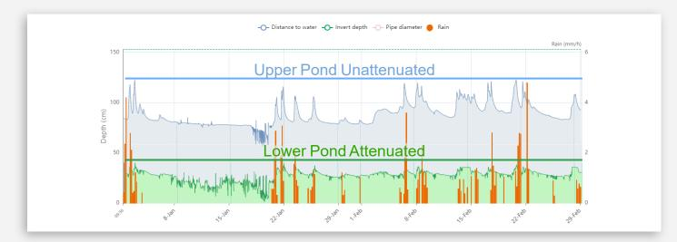
The above chart shows a typical installation at a UK Council. The Council's hydraulic engineers were able to confirm, with the data returned from the CatsEye RTU to the UDlive Portal, that the attenuation ponds performed to their design specification by attenuating peak flows in the river and providing sufficient additional storage capacity.
