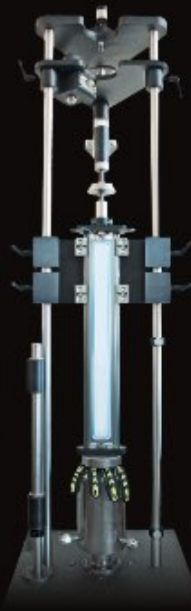
Classification for ANSI 138 Impact resistance
