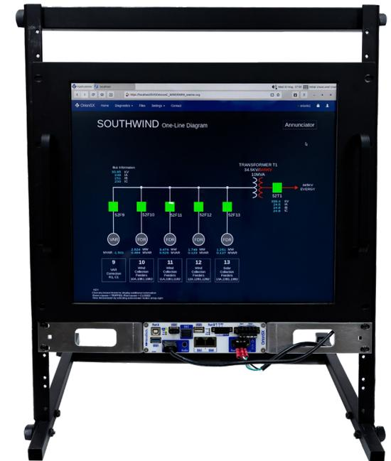
The OrionSX is ideal as a distributed HMI server, easily mounted with a monitor in multiple locations in large transmission substations. The OrionSX browser can be pointed to the substation RTU to view the same pages; no points configuration or page configuration required.
