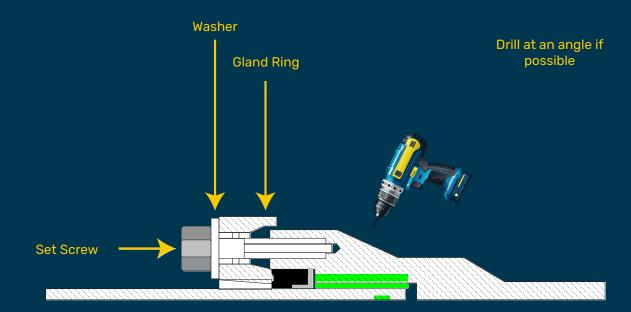
Drill at the back of the bell housing preferably at an angle Area for sealant marked in green
