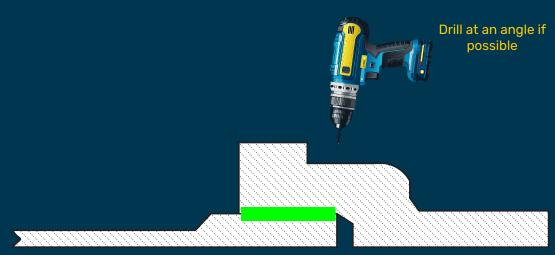
Area for sealant marked in green Drill in at the back of the socket, preferably at an angle
