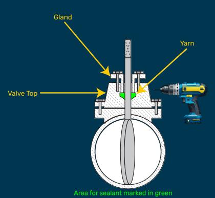
Drill into the valve top up to the yarn
