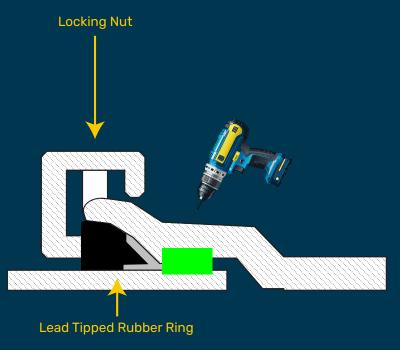
Area for sealant marked in green Drill at the back of the bell housing
