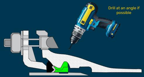
Area for sealant marked in green Lead tipped natural rubber gasket
