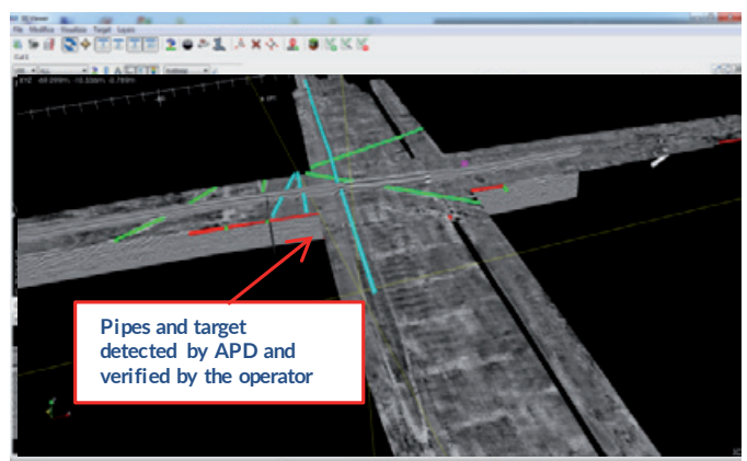
GRED HD 3D CAD: post processing software with pipe results
