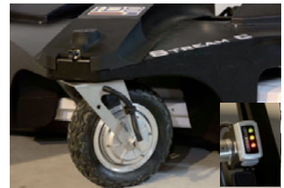
Stream C pivoting and motorized front wheel
