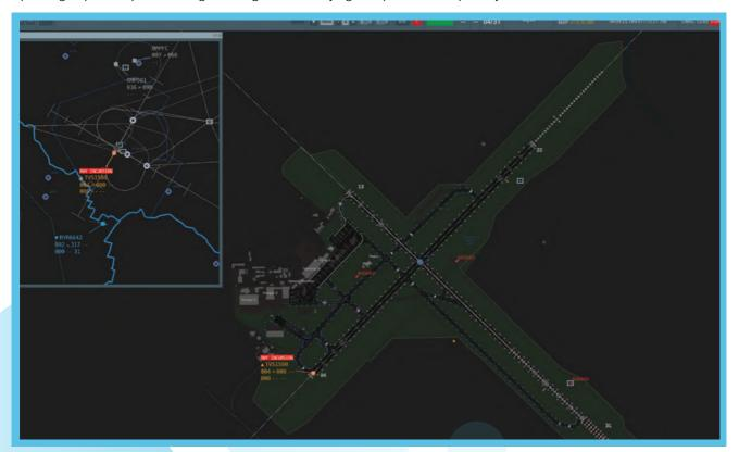
EFS module provides the user with a set of customized predictive clearances to be issued with respect to operational and safety aspects, local rules, and applied to a specific phase/type of flight or flight operation.
