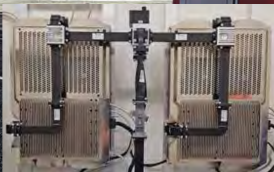
Easat Solid-State, Dual Redundant X-Band Transceiver
