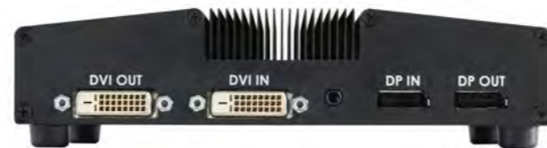
Re/Vue Pro 2 Max Single channel with DisplayPort or DVI and audio connectors
