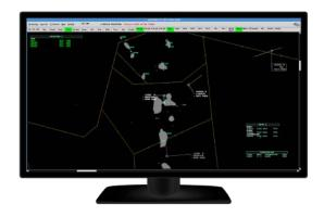
**Airspace Situation Display** for an integrated presentation of all surveillance data (ADS-B, Multilateration, Radar, ADS-C and pilot position reports).
