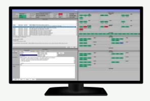
**Control and Monitoring System.** Aurora's Control & Monitoring System (CMS) capabilities include presentation of the operational status of all processors, their hardware and software components, operational status of external links and services: AFTN, SITA datalink, ADS-B & MLAT, billing, Meteorological Office and Tower systems, monitoring of Aurora system components, restarting of any failed hardware or software component, and much more.
