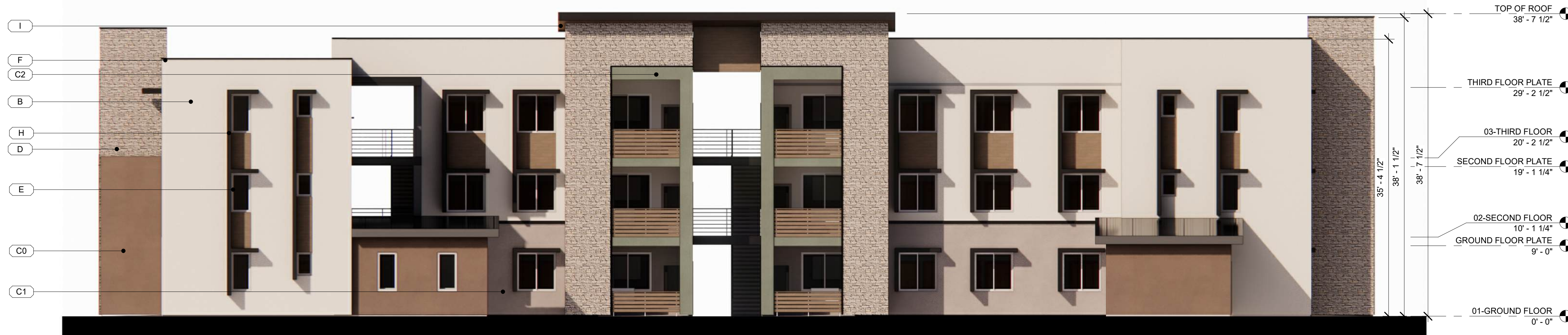
2 SOUTH ELEVATION (SIM. BLDG 4 NORTH ELEVATION) SCALE: 1/8" = 1'-0"
