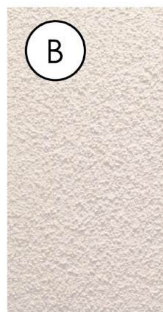
EXTERIOR PLASTER 16/20 SAND FINISH EXTERIOR WALLS LA HABRA: EGGSHELL
