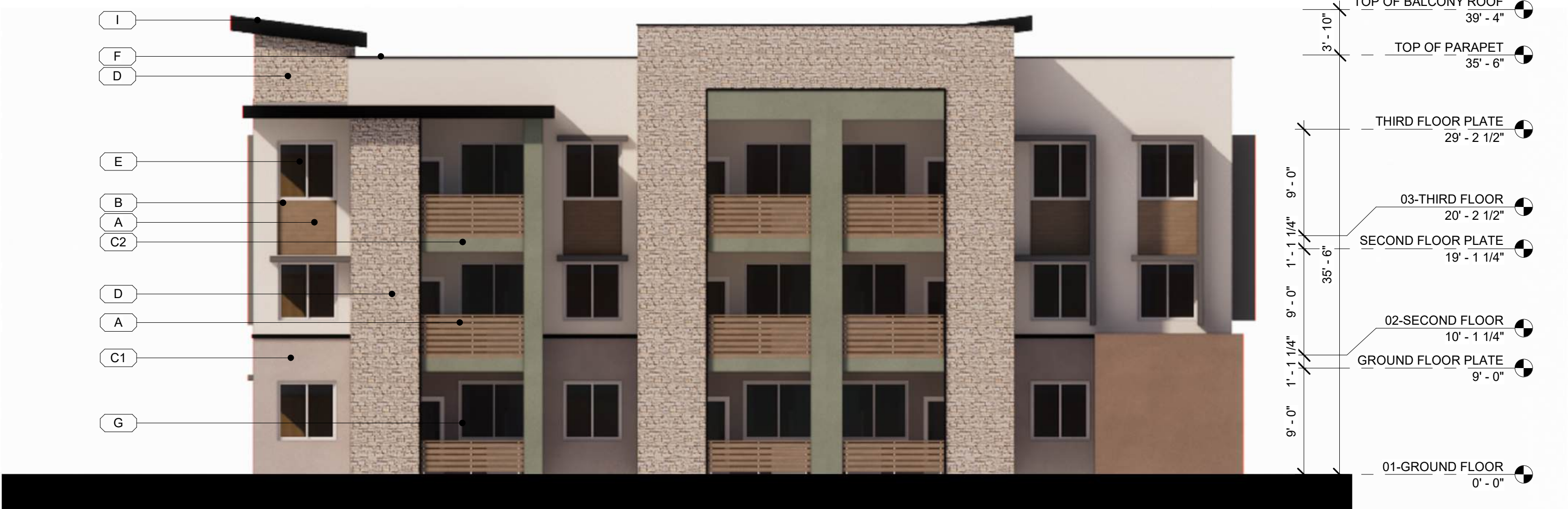
1 WEST ELEVATION (SIM. BLDG 5)
