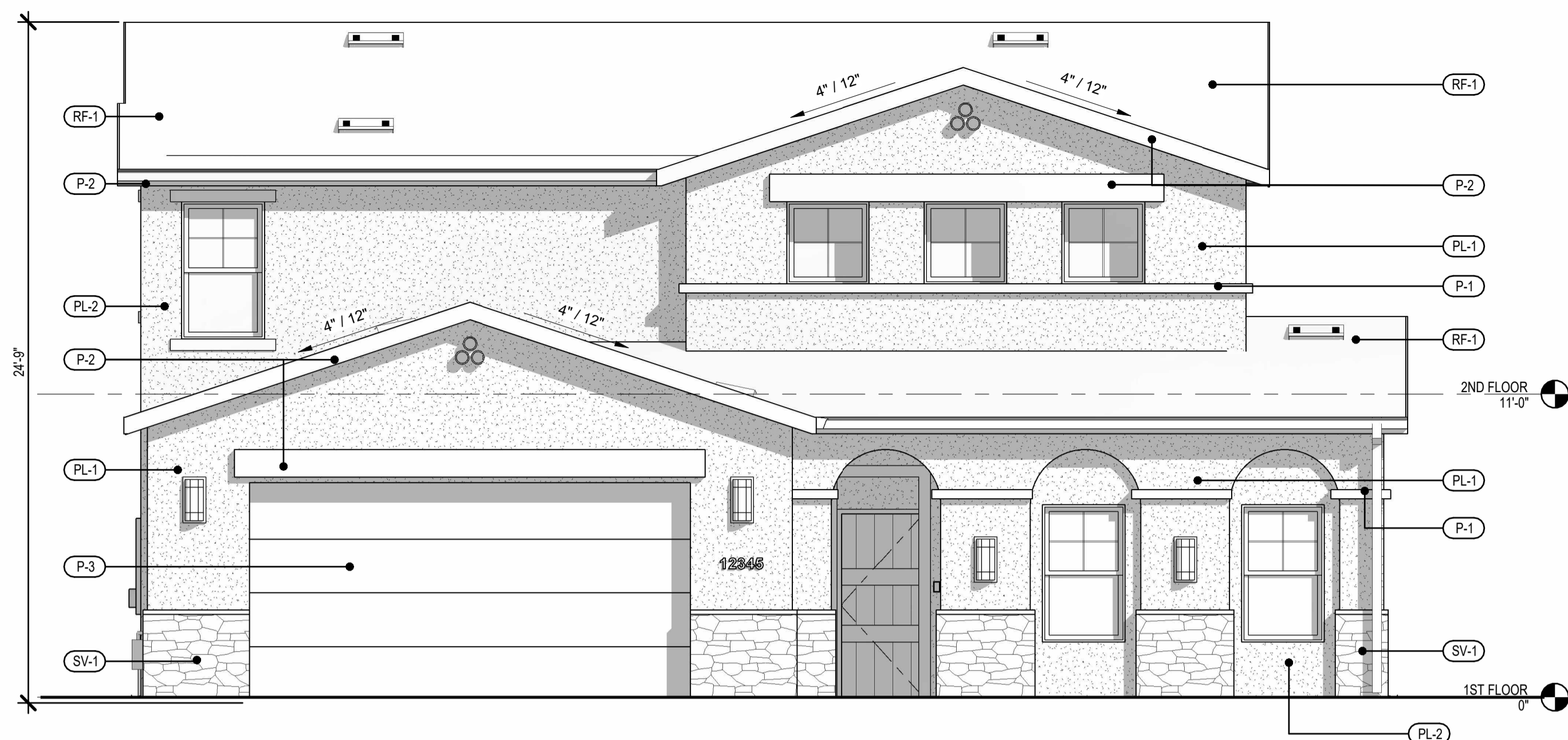
1 PLAN B - SPANISH ELEVATION - FRONT 1/4" = 1'-0"
