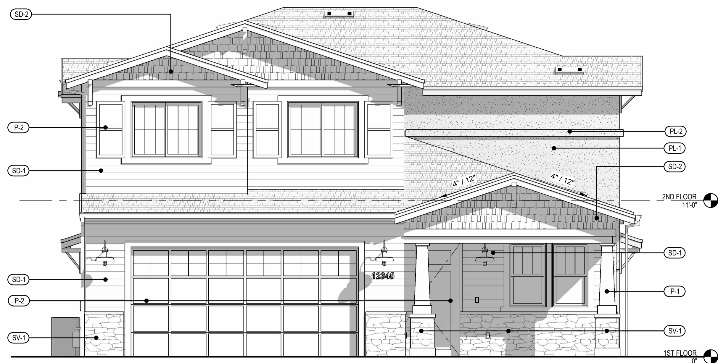
③ PLAN A - CRAFTSMAN ELEVATION - LEFT 1/4" = 1'-0"
