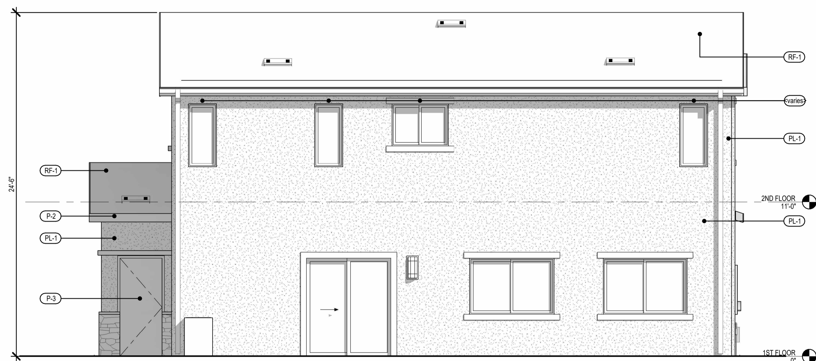
3 PLAN B - SPANISH ELEVATION - REAR 1/4" = 1'-0"
